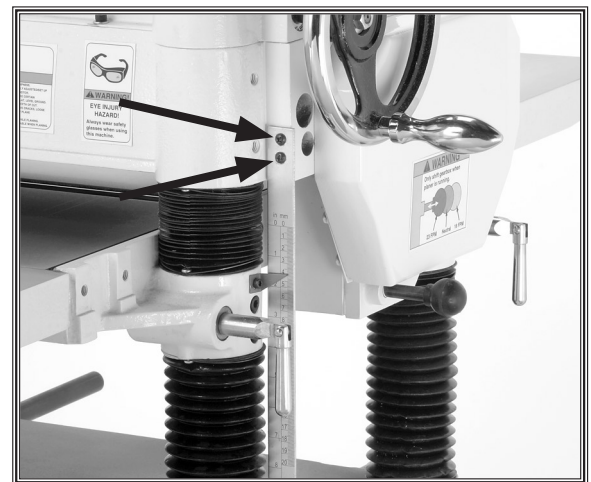
Figure 33. Depth scale adjustment screws.
